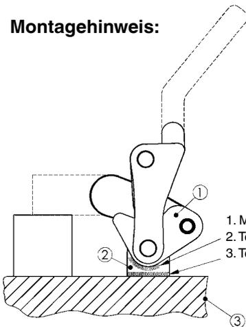
1. Modulspanner in Spannposition fixieren
